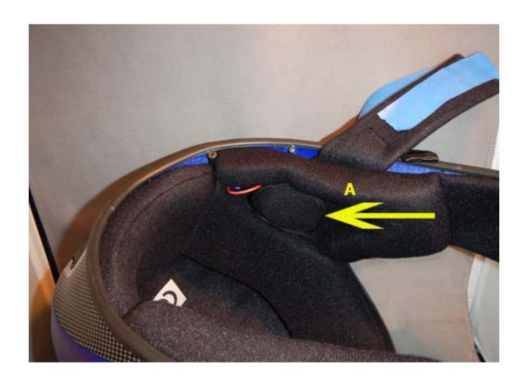
A. To complete the installation mount the right speaker as shown, on top of the ear pad. The best stereo music quality will be achieved by adjusting the speaker position to be directly over the ears.
