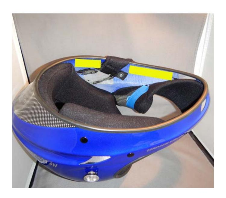
Cut two pieces of adhesive backed hook velcro and ahdere them to the helmet shell as shown. When the installation is complete this will help secure the liner to the shell without glue.
